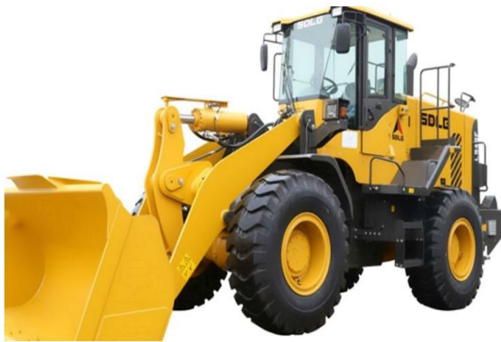
Front end Loader or Concrete Dumper: used for moving a pile of material from the ground without spreading it
