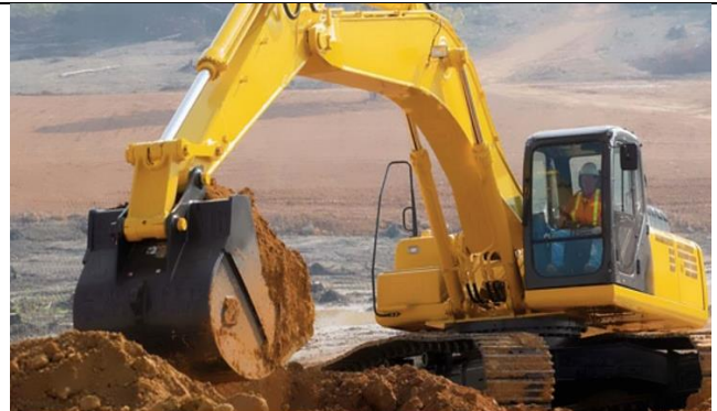
Crawler excavator: Used for excavation of earth rocks and loading them into a dump truck
