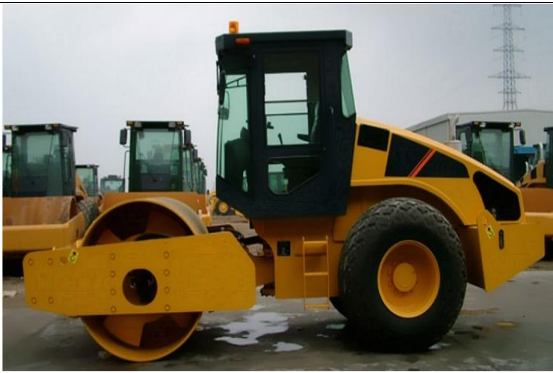
Drum Roller: Used for compacting the roadbed.
