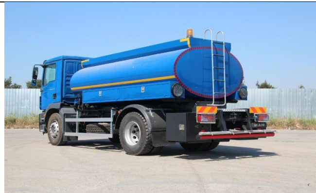
Water Bowser: to spray water on the site to reduce dust levels and supply water for concrete mixing.
